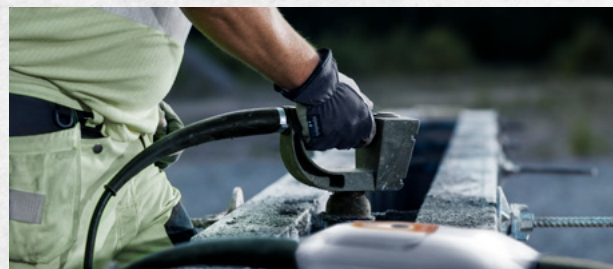
The Smart-E version features a pistol grip handle that reduces hand/arm vibration.
